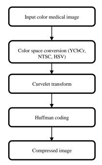
Figure 1. Block diagram of proposed system
